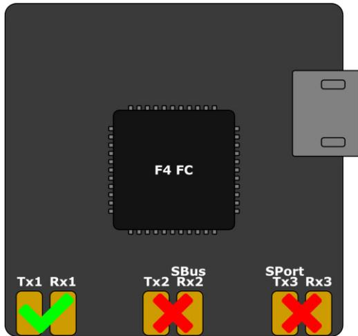
If you use a **F4 FC**, make sure you don't use UART's with labels with *SBUS* or *S-PORT*. Those UART's got a hardware-inverter installed which does not work with CRSF.
